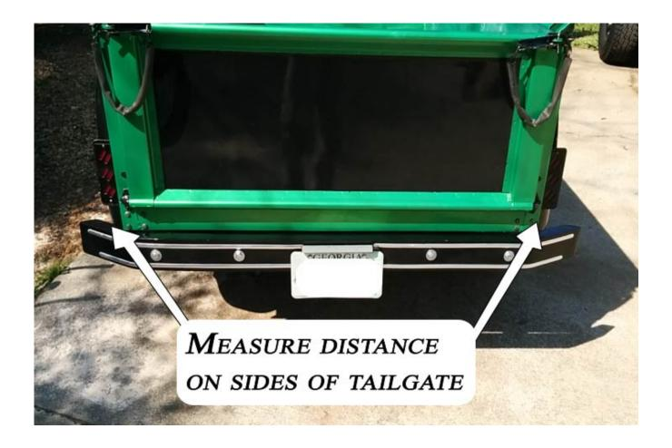
Align bumper to center of tailgate and tighten lock-nuts on bumper carriage bolts.
