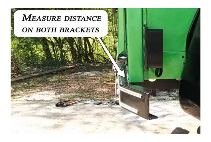
Align bumper to desired distance and tighten lock-nuts on bracket to frame bolts.
